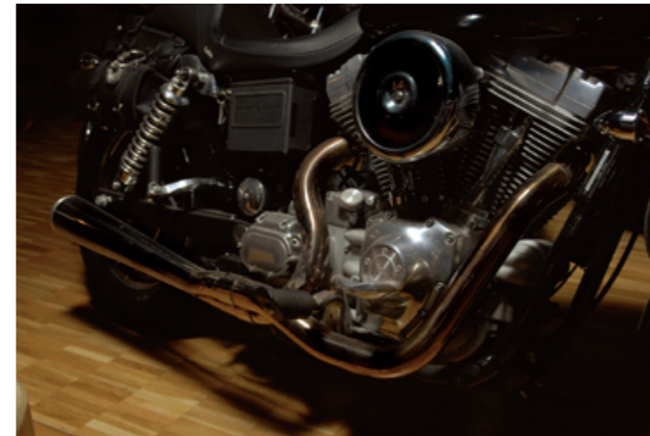
▶ Example of use of bent pipes Type: DYNA The bent pipes used in this example Front:φ50.8×30°/80°/30°/30° Rear:φ45×80°/140°
